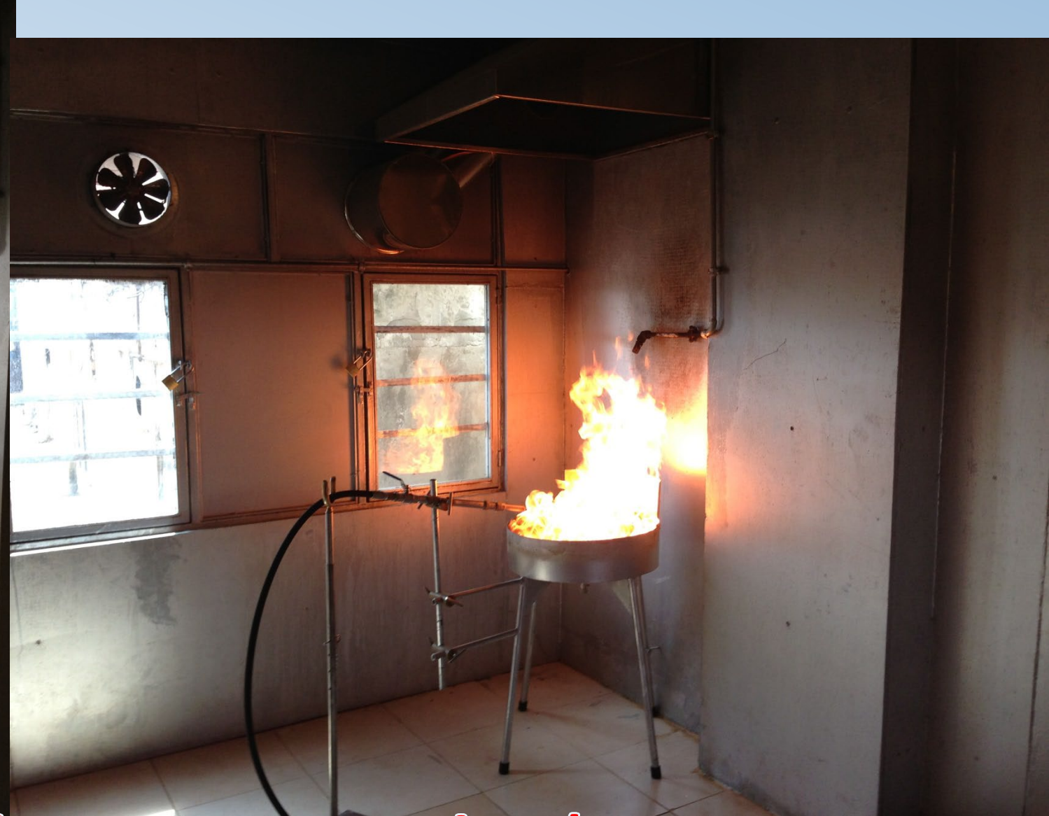
Small scale fire test for Foam samples (As per Msc 1312)
